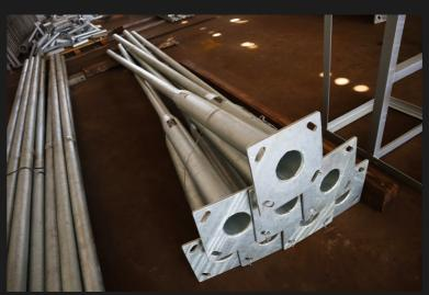
UNIK's high mast pole stands at an impressive height of 20 m. These poles are multipurpose; they function as stadium mast poles, floodlight poles, and even signage poles.
